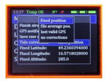
*Fixed position* – the position on the Earth is fixed to a constant value.
