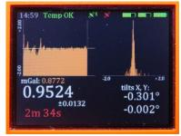
Perform gravity measurement (preset time is 3 minutes).
