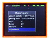
Select *Settings* from the main menu, then *Calibration* and finally *Drift* to edit the calibration.
