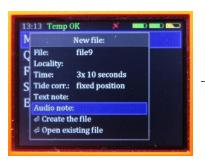
Any data file as well as any measured point can be completed with audio note. Each audio note is stored and exported as a separate file.
