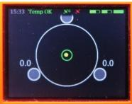
Level the probe into the green circle on the control unit's LCD. Note the probe's LCD does not indicate proper tilt at that time.
