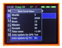
It is necessary to set proper local time. The local time is displayed on the left upper corner of the LCD as well as stored in measured data file.
