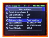
Select *Tide correction* to choose the type of tidal calculation. This will be used for initial set of tide correction when new measurement created.
