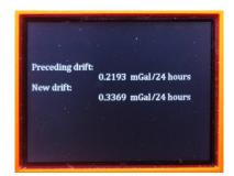
Finally confirm the drift calibration change.
