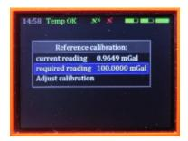
Choose option *get reading* to start gravity measurement. Once the measurement is finished the name of the item will change to *current reading*. Fill in the *required reading*.
