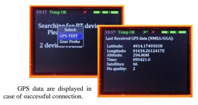
Green GPS symbol with a number of satellites is shown while external GPS data are received. No symbol means no GPS data receiving.
