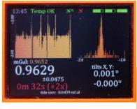
**Right arrow** to switch between graphic screen and text screen with last 5 measurements
