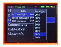
*LCD backlight* changes control unit backlight intensity. The backlight intensity can also be changed directly in any menu if you press *Enter* button longer than 1 second. The backlight intensity changes automatically as long as you hold the button.
