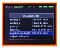
Preceding gain: 1.082298 New gain: 1.081424 Select *Settings* from the main menu, then *Calibration* and finally *Gravity* to edit the calibration.
