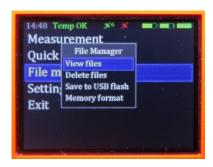
File Manager allows reviewing of measured data, deleting of useless files from data memory, saving files to USB flash disk or erasing the whole instrument memory.
