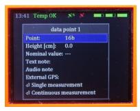
Point – label of the measured point. Automatically increased when going to the next point (e.g. label 25a is increased to 25b, label dyke59 is increased to dyke60).
