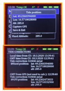
To change the fixed GPS position select *Measurement / Tide corr.: / Fixed position*. The values can be changed manually or by capturing the current position from GPS receiver.
