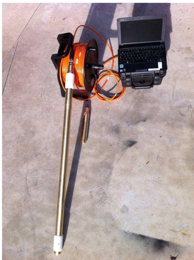
*Illustration 1: Probe with 60 m cable*
