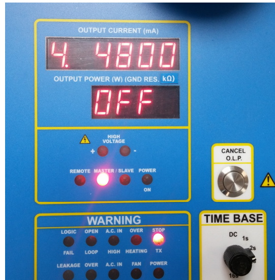
4 TX in the Multi-TX chain with total nominal output voltage of 4800V
