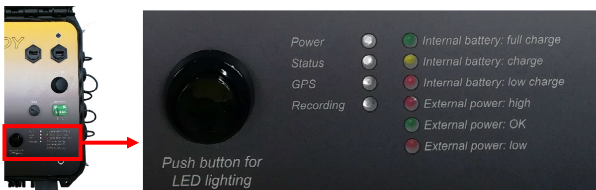
Figure 3 – Detail of the internal panel of the case that integrates the LEDs for the signals and the relative button
