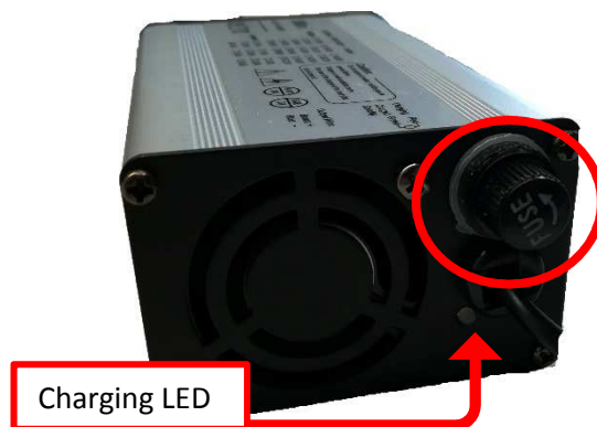
Figure 1 – Detail of the charger on the side integrating the protective fuse holder
