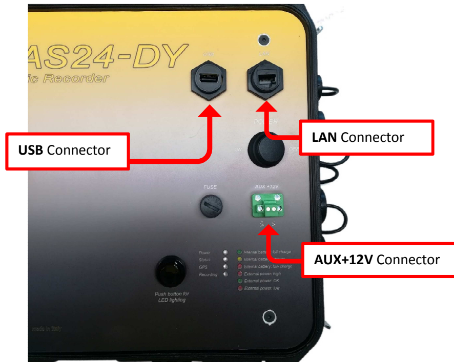
Figure 6 – Detail of the internal panel of the case integrating the connectors
